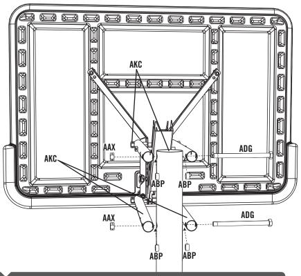
Note: Tighten the 1/2" Centerlock Nuts (AAX) until they are flush with the end of the Bolts. Make sure all hardware is securely tightened before moving to the next section.
