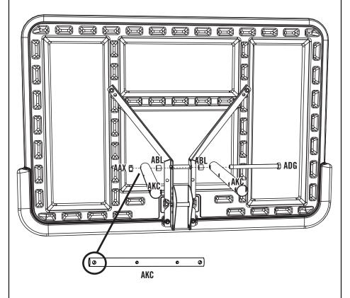
Note: Tighten the 1/2" Centerlock Nut (AAX) until it is flush with the end of the Bolt.
