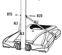
Note: Tip the system forward so the Pole rests on the ground. Do not stand the system up until it is filled with either sand or water later in the assembly.
