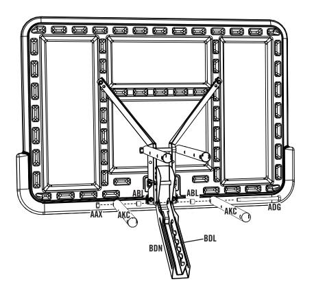
Note: Tighten the 1/2" Centerlock Nut (AAX) until it is flush with the end of the Bolt.
