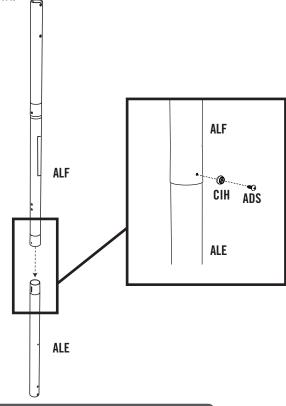
Note: The 1/4" x 3/4" Screw should be flush with the Pole, but will spin freely once installed. Do not jam the Poles together until instructed.
